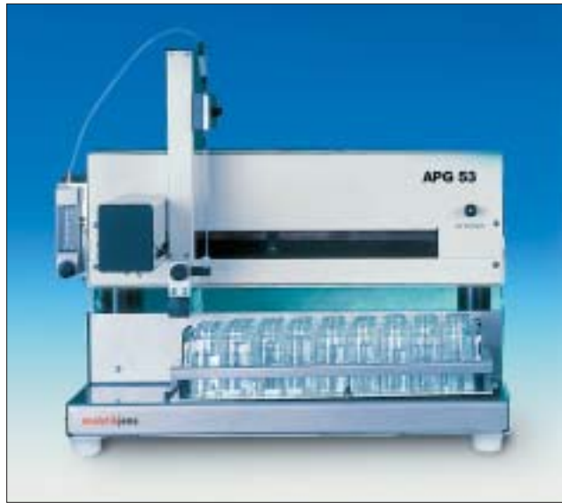
Fig.: The sipper/sampler system for automatic sample feeding consists of the xyz autosampler and a peristaltic pump
